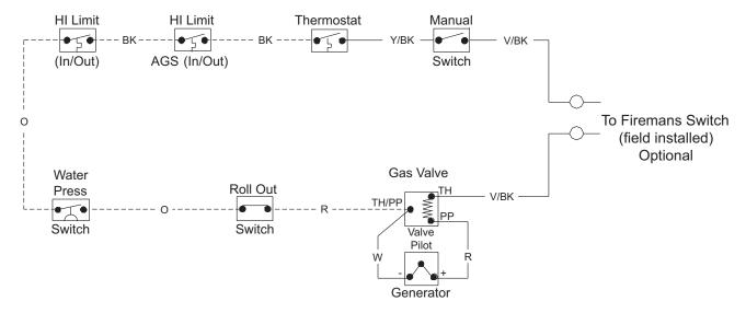
Figure 18. Wiring Diagram - Millivolt Models.
